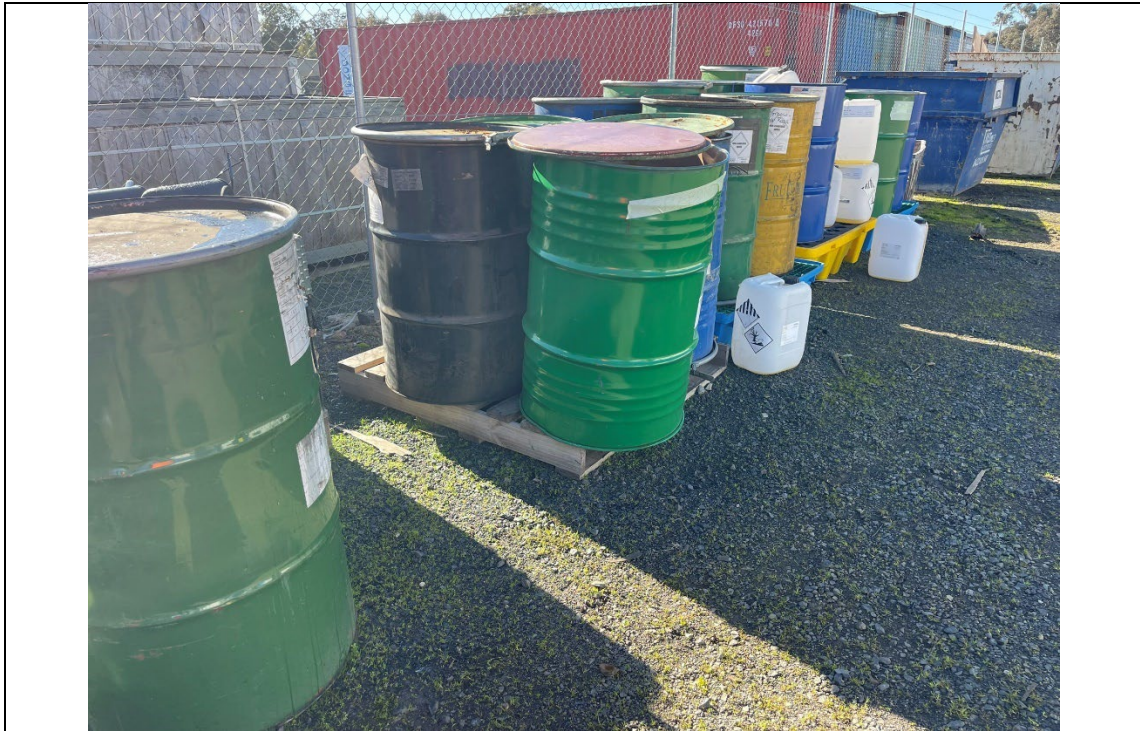
Photo 6 External waste oil storage area, uncovered. Some drums not banded.
