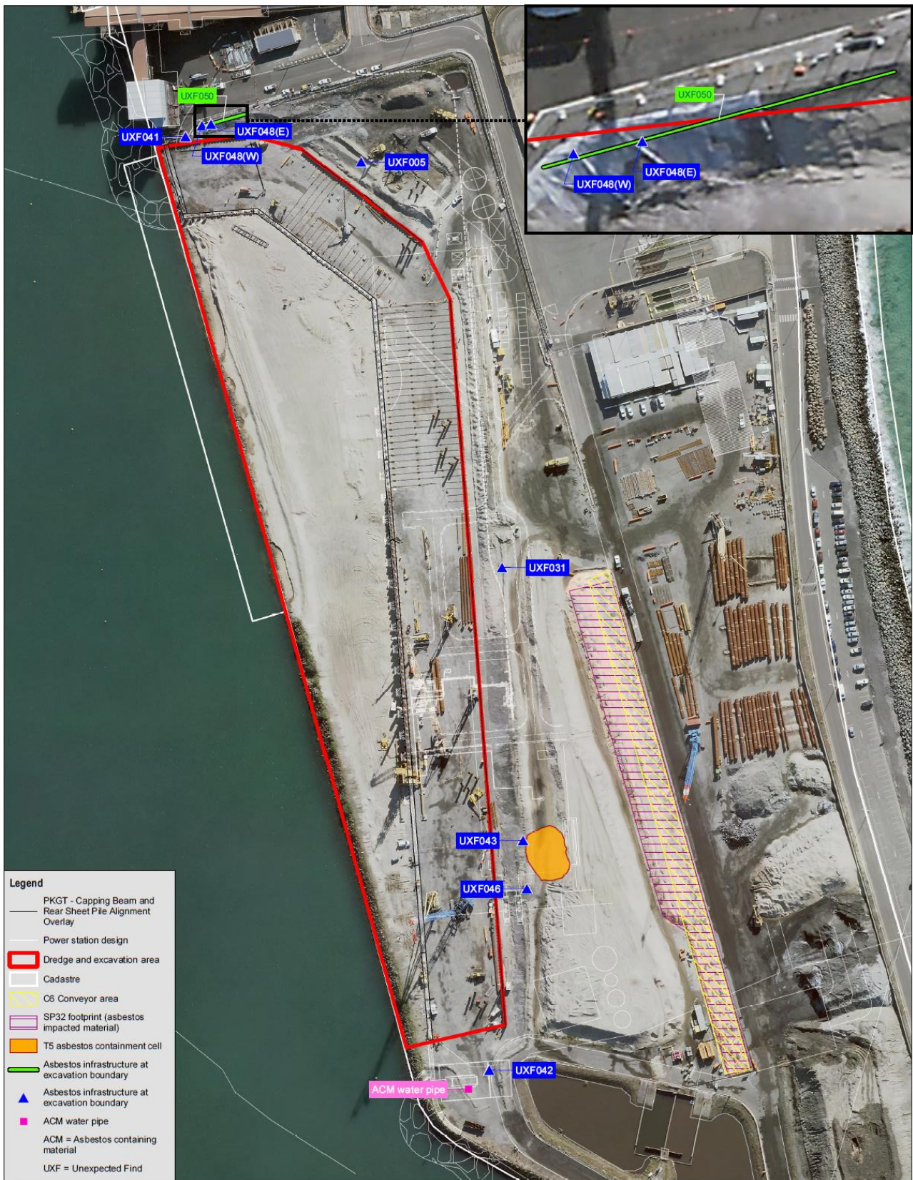
Figure 5-2 Summary of remnant asbestos remaining on site
