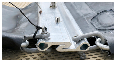
▲ The claw grip used by ASTM connectors
