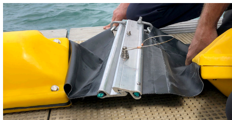
▲ Connecting pieces of boom together
