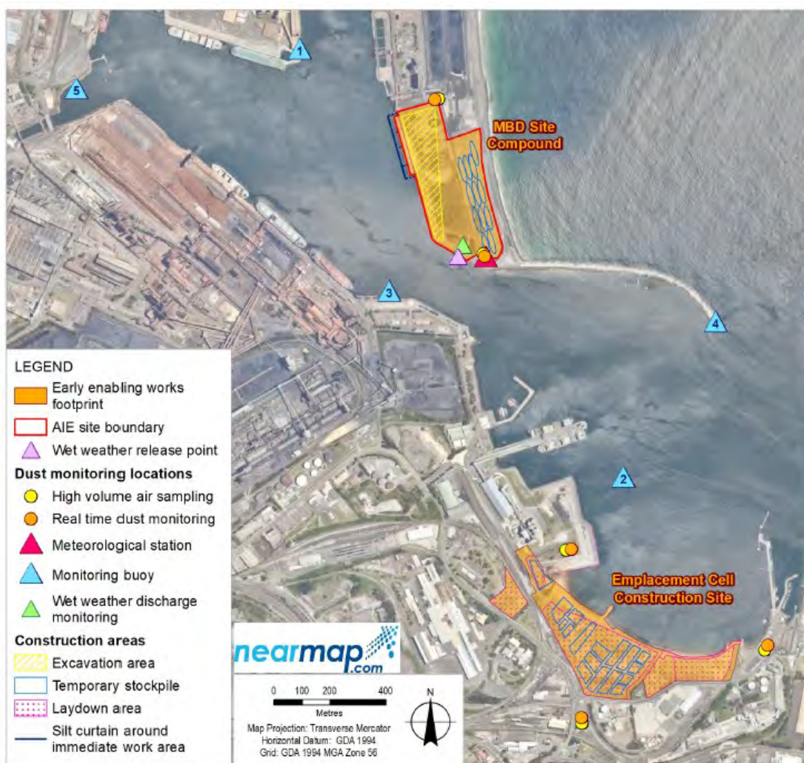
Figure 4.5 Construction Water Quality Monitoring Plan Locations
