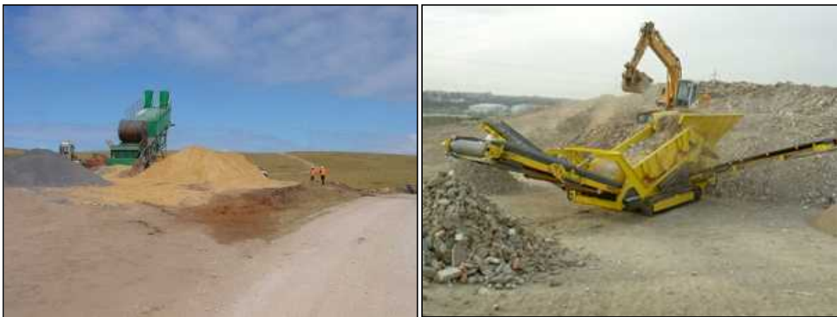
Image 3.9 Temporary on-site concrete batching plant and rock crusher
